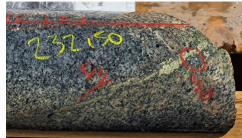
Molybdenite with chalcocopyrite indicates proximity to a porphyry core or thermal centre (DR-25-002, 232.50m)
