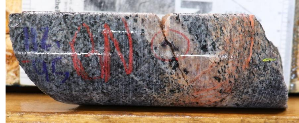
Bornite ± chalcocopyrite ± magnetite assemblages signal hypogene copper mineralization at high temperature (DR-25-001, 111.45m)
